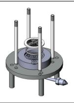
Mount the large O-ring (5) and stainless steel micron pore support plate (7) on the filter supporting base in order.
