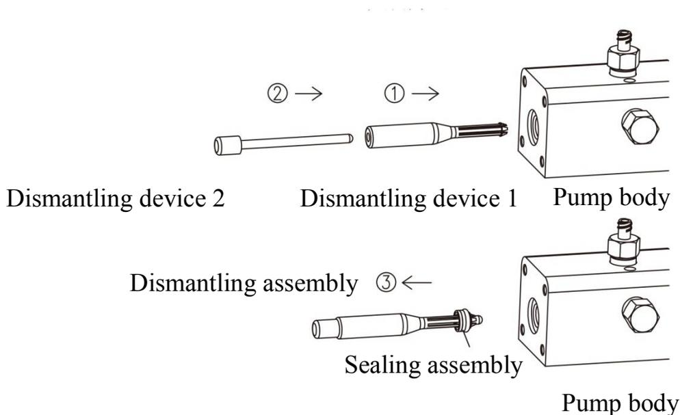
Figure 5 Dismantling of sealing parts
