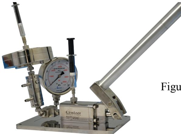
Figure 2.3 Connect with chamber and extruder
